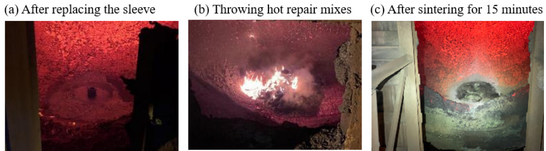
Fig.7. Application of hot repair mixes. (a) after replacing the sleeve, (b) throwing the hot repair mixes, (c) after sintering for 15 minutes.
